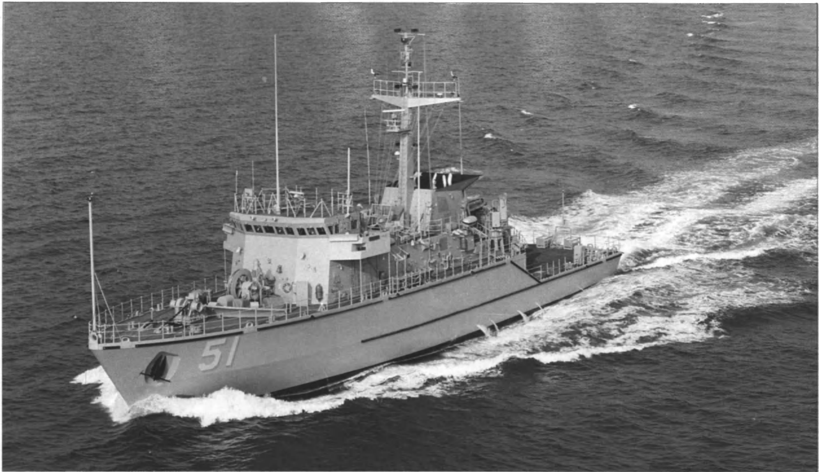
The Osprey, the first ship of a new class of Minehunters for the U.S. Navy from Intermarine USA, is constructed of glass reinforced plastic.
