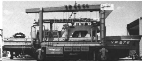
250 AMO with 108 YP Navy Training Vessel at U.S. Navy Small Craft Repair Facility, Annapolis, Maryland.
