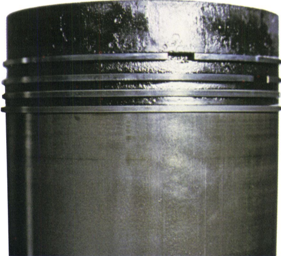
After over 23,000 hours, piston #1 of the starboard engine of an EMD 16-645 E7 shows light lacquer on skirt; rings in good condition, none stuck; only normal drag lines. Tornus Oil fights wear and lacquer buildup.
