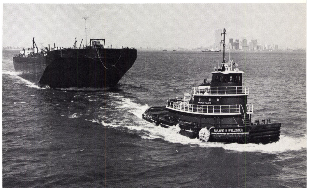
Tug Marjorie B. McAllister with barge on hawser, pilot house lowered to a conventional 28' height of eye.
