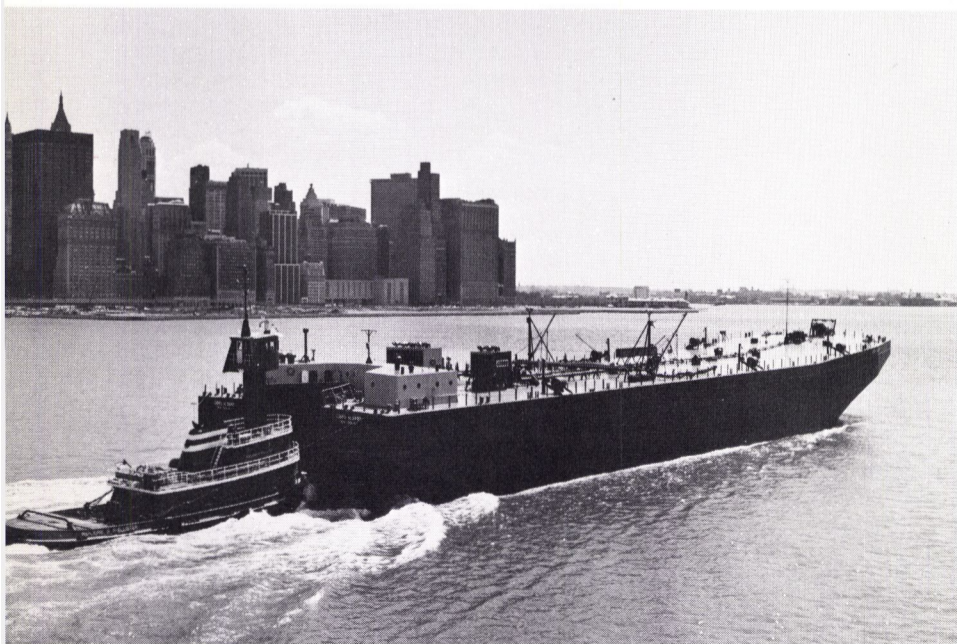
Tug Marjorie B. McAllister in notch of 18,000 ton/125,000 barrel barge. Pilot house elevated to 45' height of eye.
