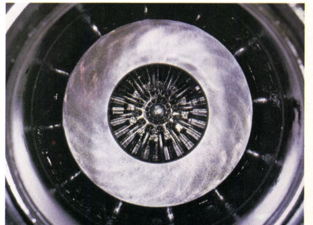
From the same engine as the wrist pin bushing, this piston undercrown is clean, free of deposits. Tornus Oil resists sludge, lacquer and carbon deposition. This promotes cooler running pistons.
