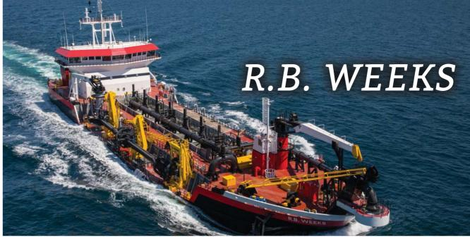
Florida shipbuilder Eastern Shipbuilding Group (ESG) this Spring delivered R.B. Weeks, a 8,550 cubic yard capacity trailing suction hopper dredge constructed for Weeks Marine, based in Cranford, N.I.
