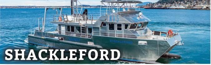
Built to service the growing offshore wind market as well as accomplish many other scientific survey missions, Shackleford is a 73- by 26.7-foot aluminum research and hydrographic survey vessel constructed by Bellingham, Wash. shipbuilder All American Marine (AAM) for the growing fleet of Geodynamics, an NV5 company.
