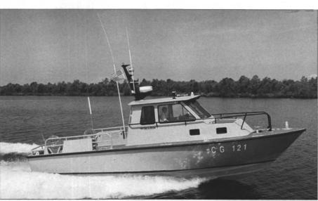
SeaArk's new Dauntless vessel is a deep vee hull design.
