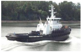
tons, the tugs are qualified to sail in all U.S and worldwide waters with the smallest possible crew. They are fitted with a pair of Schottel 1515 Z-drive units for superior maneuverability of tows in port and in close quarters. Living spaces are acoustically-dampened and fireproofed using the NORAC and Danacoustic systems, ensuring crew comfort and safety.
