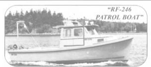
Length 25' · Beam 8' 6" · Draft 18" Displacement 6000lb · Power O/B or I/O
