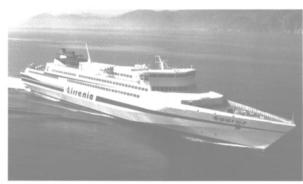
The inclusion of Fincantieri on the Lockheed Martin-led LCS team means the delivery of high-level commercial success in the realm of big, fast craft. Pictured here is Taurus, a ferry powered by a pair of MTU diesel engines and a pair of General Electric gas turbines.
