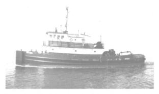
the hull and deckhouse modification. Two CAT 3512 engines and 4:1 Twin Disc gears will power the tugboat. Two 65kW generators will supply the ship's service power.
