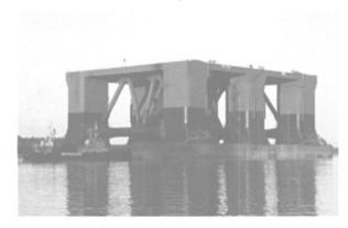
The multi-purpose bare-deck platform CS50 represents the fifth generation of semi-submersible platforms designed by Moss Maritime AS (Norway). The platform, which measures 389 x 231 x 133 ft. (118.6 x 70.4 x 40.6 m) with a hull weight of approximately 15,000 tons, is of a catamaran type with two pontoons and six stabilizing columns supporting the upper structure.
