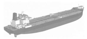
Seahorse Shuttling and Technology LLC, a wholly owned entity of Conoco, has completed the functional design of a new tanker for shuttling crude oil from the deepwater Gulf of Mexico to shore. The 80,000-dwt double-hulled "GoMAX 550 shuttle tanker will be capable of transporting 550,000 barrels of crude oil. With a 40-foot draft, the new shuttle tanker will be able to enter most ports in the U.S. Gulf of Mexico.
