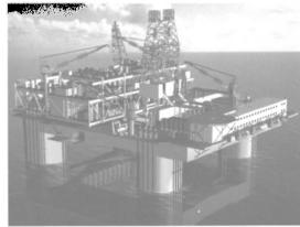
will be produced using the "Thunder Horse PDQ" platform. Displacing 129,000 tons, this will be the largest semi-submersible production platform in the world. It will be delivered from Korea in 2004
