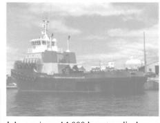
July, towing a 14,000 long ton displacement combination railcar/container barge between Seattle and Whittier, Alaska. Propulsion power comes from two Cat 3516B High Displacement marine diesel engines supplied by N C Power Systems, Seattle. Each electronically controlled Cat engine is rated 2,260 bhp (1,686 bkW) at 1,600 rpm, and drives an Ulstein Z-drive with Nautican propeller and nozzle.
