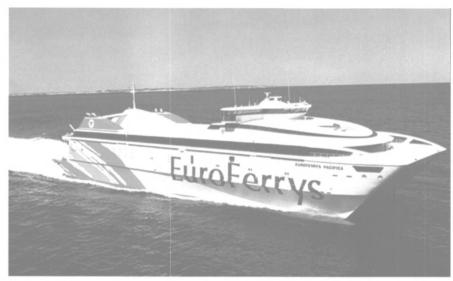
Euroferrys Pacifica has a passenger capacity of 951 passengers and 251 cars. Its propulsion package comprises 4x Caterpillar 3618 engines, 4x Reintjes geaboxes and 4x Kamewa 125 SII wateriets
