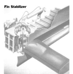
Fin Stabilizers - By using airfoil-shaped fins mounted low in the hull amidships, significant roll reduction can be achieved when the vessel is underway. Such fin stabilizers use a motion sensing controller that signals the fin to change its angle of attack to the water, thus producing a countering force to the wave motion. Fin stabilizers are typically electrohydraulic units and are more effective the faster the vessel is moving.
