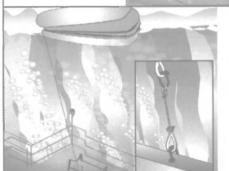
As the vessel sinks, the painterline will be stretched and the liferaft starts to inflate.
