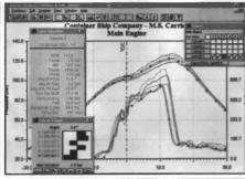
electronics which has designed to allow the user to take engine readings and see calculated realties without having to interface to a PC at any stage. The instrument is still able to display the plot of pressure versus angle, but in addition has tabulated results for multiple cylinders including Pmax, angle of Pmax, power (in kW and hp) and the maximum rate of change of pressure.
