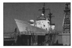
Bellingham Bay Shipyard recently completed a pair of U.S. Coast Guard repair contracts worth \$2.8 million for the 378 ft. (115 m) cutters Mellon and Midgett. In addition to maintenance and voyage repair work, both projects involved drydocking, complete blasting and painting of freeboard and underwater body, rudder bearing replacements, and cooler and piping renewals on the ships' supplementary gas turbine engines.
