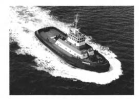
The tractor tug NAMAHOE, now in service in Hawaii; 4,400 HP with twin Z-drives: 105'  $\times$  34'  $\times$  16.5' (32  $\times$  10.4  $\times$  5m).
