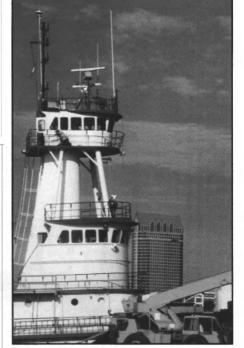
Maritrans innovative barge rebuild program didn't stop with the barge. The upper pilothouse for the tug will now be the primary steering station, so it was enlarged for comfort and also raised
