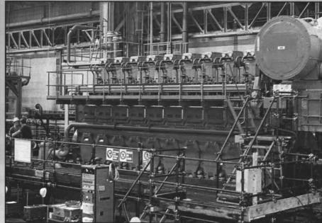
The ZA50S engine, one of two nine-cylinder units for the first Tor Line RoRo newbuilding at Fincantieri
