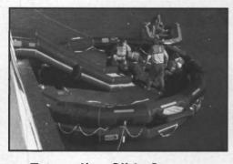
Evacuation Slide System. Designed specifically for Low Freeboard Vessels, it is a combination slide and platform. It provides speedy evacuation for all passengers voung, old and physically challenged. US Coast Guard Approved.
