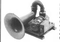
Model S-120 Piston Horn Chosen for use on aircraft carriers as well as commercial vessels over 200 meters in length, the S-120 utilizes an oscillating piston driven by 7-1/2 horsepower 3 phase 220/440 volt electric motor producing 143 dB and a fundamental frequency of 94 Hz in 1/3 octave band at one meter.
