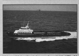
With a 30-ft. (9-m) beam, four V-12 KTA 38 Cummins engines easily fit across *Paula Kay's* engine room. Diamond Services put the 170-ft. (51.8-m), Hamilton jet-powered boat into service in Gulf of Mexico offshore oilfields in June. (photo credit: Skeets Photo)
