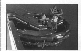
**Evacuation Slide System.** Designed specifically for Low Feeboard Vessels, it is a combination slide and platform. It provides speedy evacuation for all passengers - young, old and physically challenged. US Coast Guard Approved.
