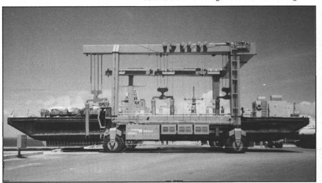
A large barge is hauled by Marine Travelift 300 BFM mobile boat hoist at a US Navy installation, Guantanamo Bay, Cuba.
