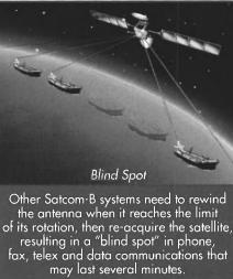
Common to most other Satcom-B systems, "antenna rewind" interrupts the critical communication satellite link, creating a "blind spot" in your vessel's voice, fax, telex or data traffic
