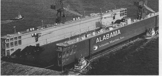
The ALABAMA has a lifting capacity of 250,000 DWT or 50,000 tons displacement. • Normal maximum draft over six-foot keel blocks is 32 feet.
