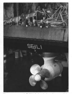
The prototype 1.5 MW Azipod electric propulsion drive on the supply vessel Seili. The Azipod will be offered in power ranges up to 20 MW.
