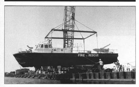
The new New York City Fire Department SES fireboat John P. Devaney being lowered into the water at Textron Marine Systems.
