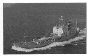
The Japan-Tuna No.3, built by Hitachi Zosen's Ariake Works for the Japan Tuna Fisheries Co-operative Association. She is designed to serve as a replenishment vessel for the Japanese Pacific tuna fleet.
