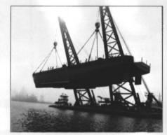
The hull of the 210-foot Louisiana Responder being lowered into the Mobile River by Bisso Marine crane barges. The oil spill recovery vessel is one of four under construction at Bender Shipbuilding & Repair Co. Inc., in Mobile, Ala.
