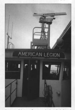
Antenna of the new Furuno radar installed aboard the Staten Island ferry American Legion.
