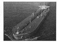
Designed to carry 2 million barrels of cargo oil and cruise with minimal resistance and fuel saving, the 1,076-foot-long by 187-foot-wide tanker Sawako has a new simplified hull structure that eliminates the center girder.
