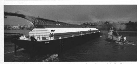
The barge ST44, built by Zidell Marine, will be used for transporting grain on the Columbia River system.
