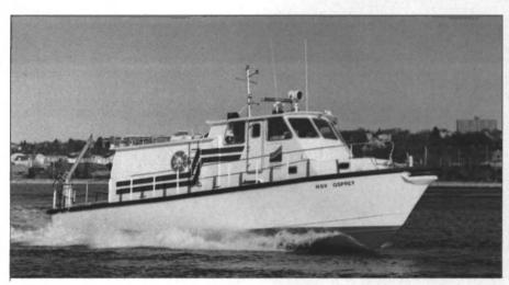
The HSV Osprey is powered by twin Detroit Diesel engines coupled to ZF reduction gears. The vessel's interior comfortably accommodates six crew members, including the captain and a mate
