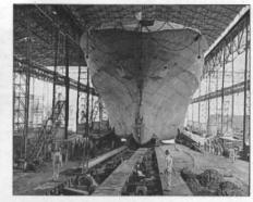
The Del Monte Quality being launched into the Guadalquivir River from the roofed yard at Astilleros Espanoles, Seville.
