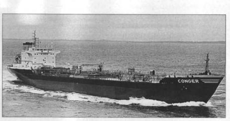
The transportation of five different, fully segregated cargoes is possible at the same time on the chemical tanker Conger, recently delivered by Lindenau.
