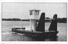
Fleet repair vessel, built by Marine Inland Fabricators, is powered by a single GM 6-71 Detroit Diesel engine.
