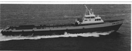
The 160-fo at crewboat Deanne McCall is powered by six Cummins diesel engines to a speed of 24 knots.
