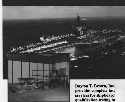
accordance with MIL-S-901 Shock, MIL-STD-167 Vibration, and MIL-E-16400 test requirements.
