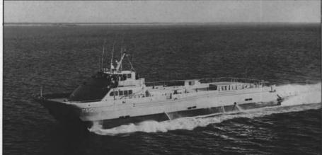
of 40 knots, following her conversion, modification and upgrading at Textron Marine Systems' style rigid sidenulis. The SE-200 was awarded to Textron Marine Systems by the U.S. Army Corps of tween the sidehulls and flexible bow The SES-200, the U.S. Navy's only Surface Effect Ship, is now able to reach speeds in excess
