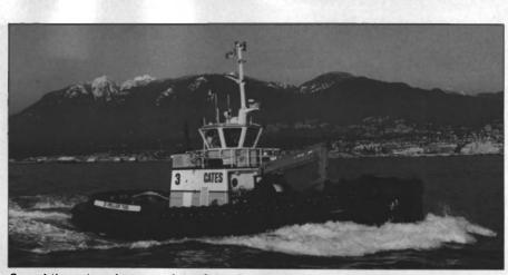
been refined through three vessels pair of CAT 3512 TA diesels, each pling. The Cates 3 is essentially identical to other Z-drive tugs in the Cates
