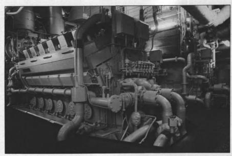
A large father-and-son arrangement. Two shaftlines with one eight-cylinder and one 12cylinder Wartsila Vasa 32 engine, totaling 22,200 bhp RCCL's Nordic Empress. The auxiliary machinery consists of the same type, three Wartsila Vasa 8R32 generating 10,320 kw.
