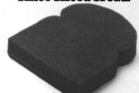
Soundcoat's exclusive SOUNDMAT PBM is made with a sheet of thin flexible limp mass sandwiched between two layers of foam to provide absorption, transmission loss and isolation. It has excellent resistance to oxidation, UV light and weathering.
