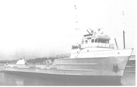
Two 900-hp GM engines and a Murray & Tregurtha bowthruster enhance the Tara Alyene's station-keeping capability.
