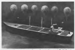
Unique salvage system shown by students at Gulf Section spring meeting uses 800,000 plastic balls pumped into the holds and six nets attached to a sunken 600-foot ship to provide negative buoyancy to raise the ship for towing.
