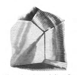
Flat-membrane design tank of Invar alloy.
