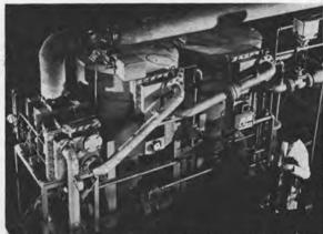
A Weir remotely controlled MXFR two-stage flash distillation plant on test at the Cathcart plant in Glasgow.
