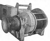
24 - American Hoist & Derrick Company Cargo Winches, 12-R.H., 12-L.H., single drum, single gypsy, Mfgs. No. 67696, rated 7400 lb. line pull at 220 FPM, total stowage capacity 709' of 7%" wire rope, powered with Westinghouse Motors, 50 HP, 230 volts DC, 600 RPM, compound wound, Type CK, Frame 9, complete with Control Panel, Resistors and Master Switch. All units are of Recent Manufacture.
