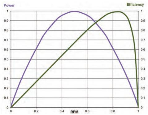
As you can see from the representative motor curves of shaft power and electrical efficiency versus RPM, the highest potential power rarely (if ever) occurs at the highest electrical input efficiency.
