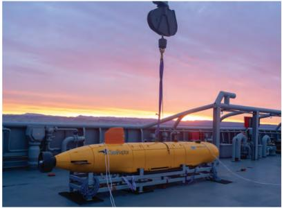
**Teledyne Gavia will introduce its new 6000 meter rated AUV, SeaRaptor** at Ocean Business in April. "In SeaRaptor, the Teledyne Marine team has introduced a high performance AUV capable of carrying the most advance marine sensors available in the market. We have already delivered our first vehicle and see significant opportunities for SeaRaptor," said Thomas Altshuler, VP and Group GM for the Teledyne Marine Vehicle group.
