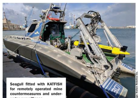
water surveillance. Kraken Robotic Systems completed a series of sea tests of its KATFISH towed Synthetic Aperture Sonar system with Elbit Systems, an international de-
